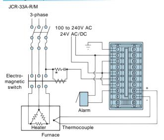
\* Surge absorber: To prevent the unit from harmful effects of unexpected level noise, it is recommended that a surge absorber be installed between the electromagnetic switch coils.
