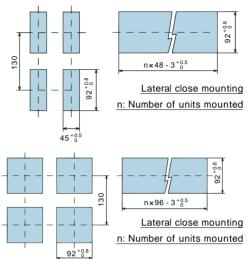
Caution: When Lateral close mounting is applied, Dust-proof and Drip-proof specification is not fullfilled.
